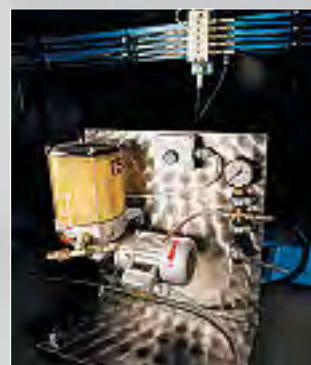
Central lubrication system with progressive distribution
