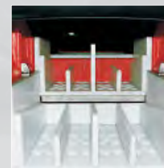
Reversing stage separation with special screen for complex part shapes
