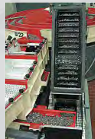
Chip conveyor system
