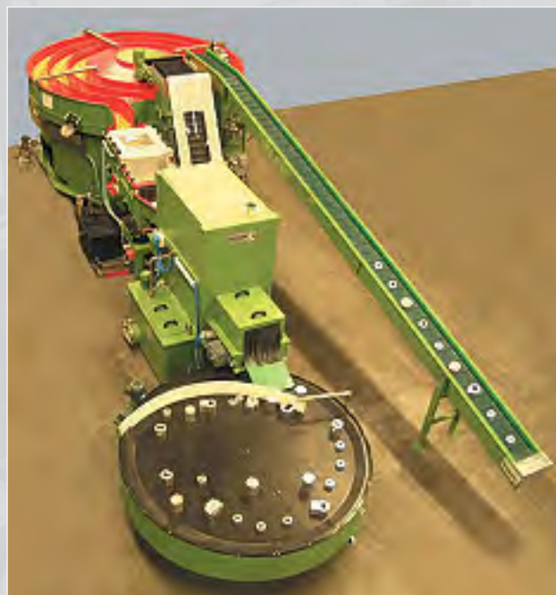
Multi-Channel machining centre for hydraulic components with loading conveyor, washer and round storage table
