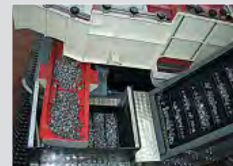
Lower cross-conveyor channel with residual water screen segment and chip conveyor belt
