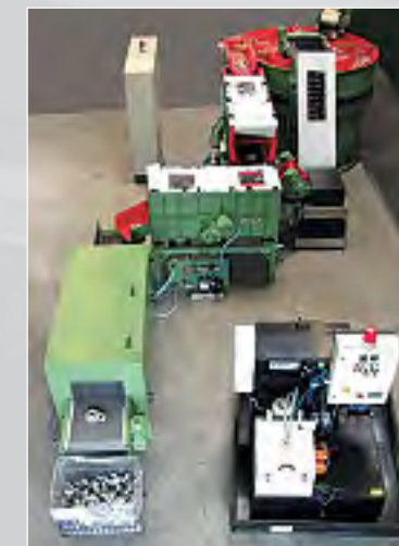
Multi-Channel system with part cleaning stage, drier and process water recycling unit
