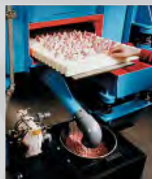
Abrasive media fines separation with collecting zone
