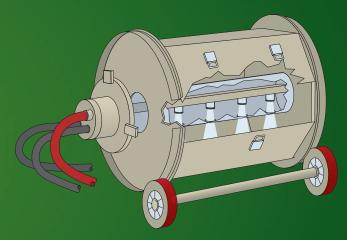
ZERO offers tumble barrel cabinets with suction blast systems only. Inside the barrel, the parts ride on a cushioning layer of media, while two to six automatic blast guns thoroughly clean, etch or shot peen their surfaces. The inside barrel is comprised of replaceable rubber covered metal panels.
