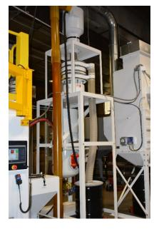
**Pressure Blast Generator** - The abrasive blasting media is fed into the compressed air stream from a six cubic foot capacity pressure vessel. Includes an Electronics, Inc., MFD-P1 Sensor for monitoring of abrasive media flow, a Proportion-Air air volume booster with electronic air pressure regulator for air pressure, and media level sensor.
