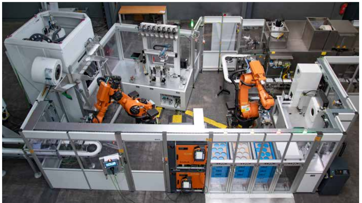
Fully automated processing line with a Rösler Multi-Surf-Finisher and a Rösler continuous flow washing system.
