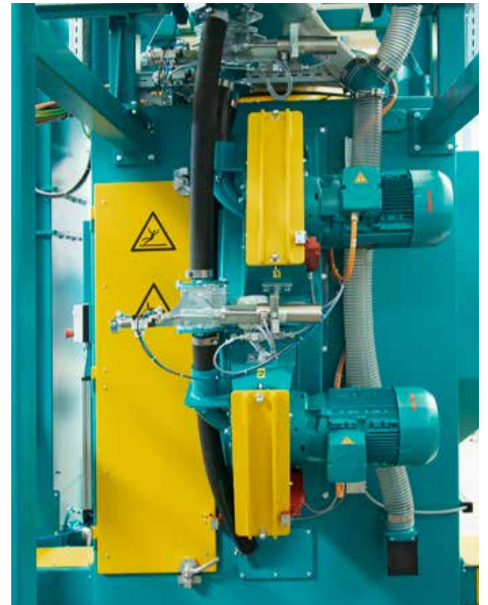
Turbine technology of the swing chamber blast machine
