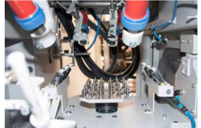
Detail of work piece fixture
