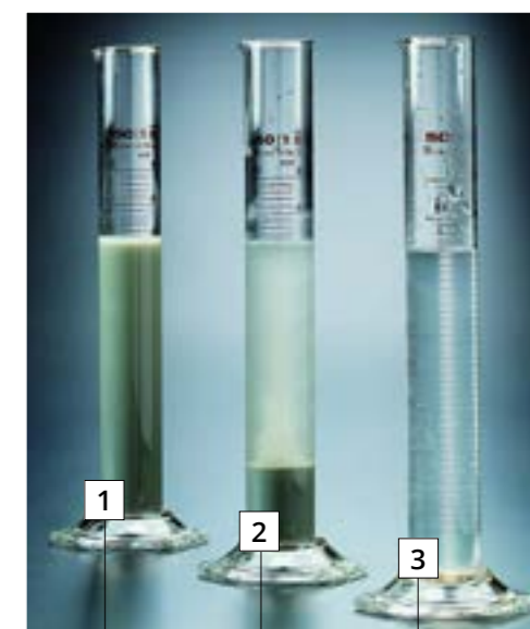
Process water after addition of process water cleaner - (The solid particles now combined into larger "flocs" are easier to separate and precipitate.)
