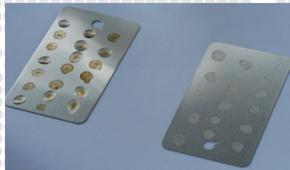
Drop test with tap water on left, panel on right treated with solution of AxxaWash™ NW-10C in tap water
