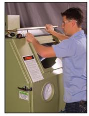
The top-mounted light module features an abrasive-resistant Lexan® cover and twin fluorescent bulbs
