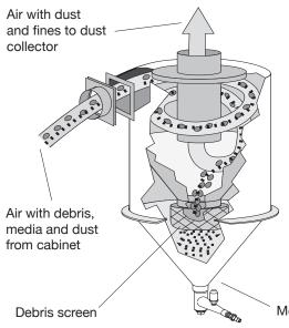
The heart of every Pulsar® cabinet is the proven ZERO reclaimerwhich efficiently separates dust and debris from reusable media. The reclaimer incorporates a wear-plate which protects the inlet from damage by debris. The large basket beneath the reclaimer screens out oversize material that can clog the blast system. A fully adjustable metering system delivers as much or as little media as needed.
