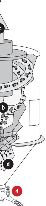
The media reclaimer maintains an effective media working mix while simultaneously removing dust and debris from the blast system. This process ensures consistent blasting results and peak blast system performance.
