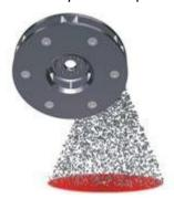
When wear occurs such as the thinning of the blades / vanes or a widening of the aperture in the impellor, the difference in the blast pattern can quickly exceed a change of 20%. This will lead to an increased blast cleaning time, decreased production output and unnecessary wear to the blast chamber. This condition leads to greater abrasive usage caused by the blast stream
