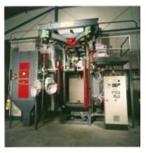
It is critical you maintain a balanced abrasive particle size to obtain a consistent, quality finish. When a machine is first installed it should be filled with new abrasive constituting a "working mix" of different sizes of media.
