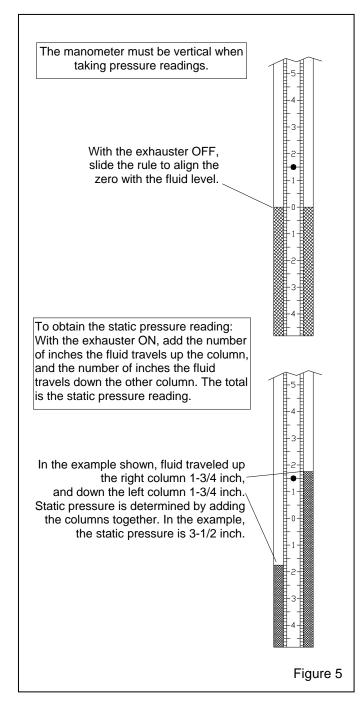
**4.1.11** After the readings are taken, replace the needle protector. Close the manometer valves and store the
