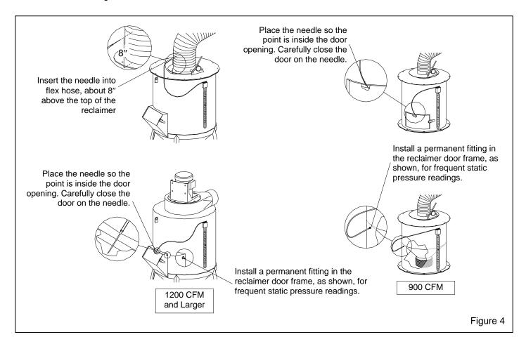
**4.1.9** Turn the exhauster ON. The negative (static) pressure will move fluid in the tube.
