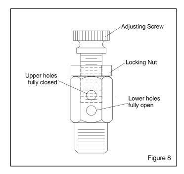
**5.4.4** If media flow is too light, decrease air in the mixture by turning the metering screw in (clockwise when viewed from the top) covering more of the holes so less air enters the media hose. Tighten the locking nut finger-tight to maintain the setting.
