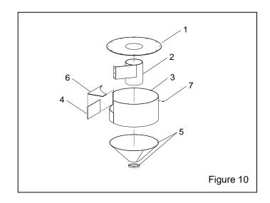
To distinguish 1200 cfm reclaimers for replacement liners, measure the distance between the bottom outside edge of the door housing and the top of the taper (not the flange), as shown below.
