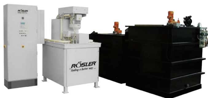
Z 1000 – fully automatic process water recycling centrifuge
