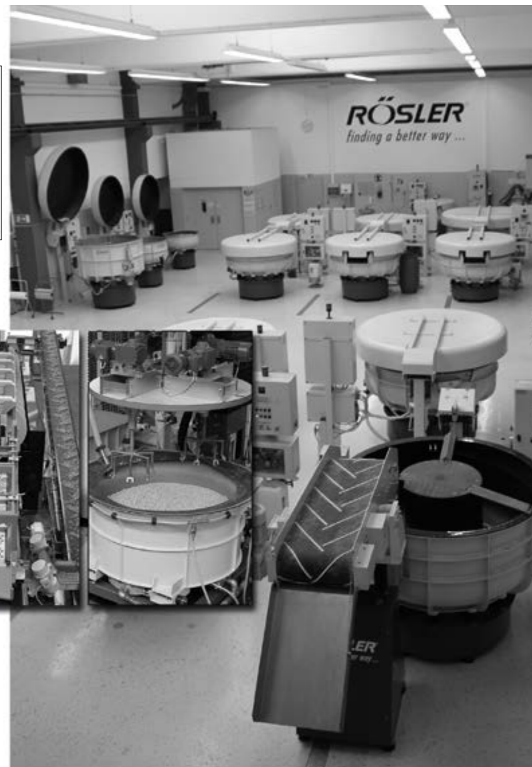
Test lab mass finishing
