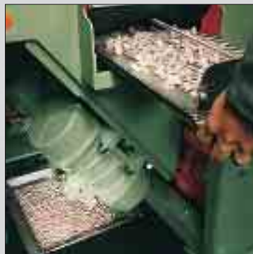
Undersize media classification with collecting bin
