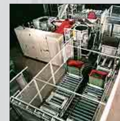
Profi-Line with parts loading system, vibratory hopper with weighing cells, rotary dryer and automatic transfer of finished parts
