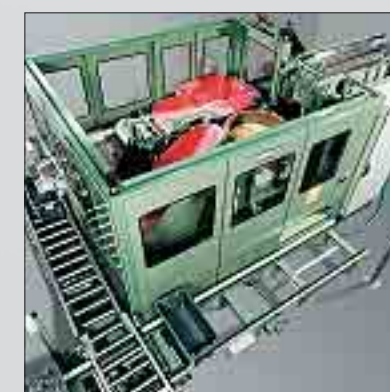
Profi-Line with vibratory hopper with weighing cells, roller conveyor and buffering of finished parts
