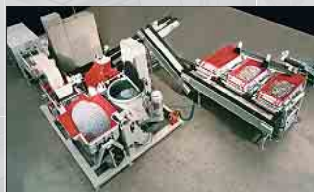
Profi-Line with 3 buffer units for raw parts, magnetic separation and hot air belt dryer
