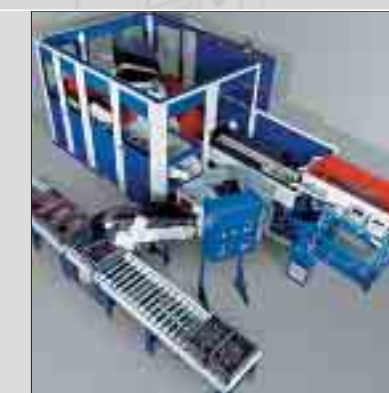
Profi-Line with vibratory hopper with weighing cells, conveyor belt, drying of finished parts in rotary dryer and roller conveyor with weighing cells
