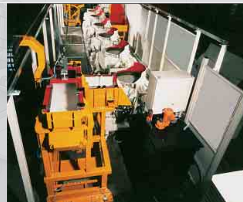
Multiple stand-alone centrifugal disk finishing machines with automatic parts loading and unloading
