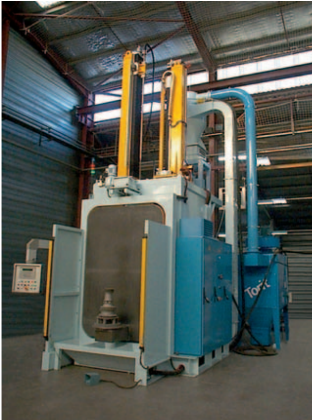
Surface preparation for compressor and turbine shafts
