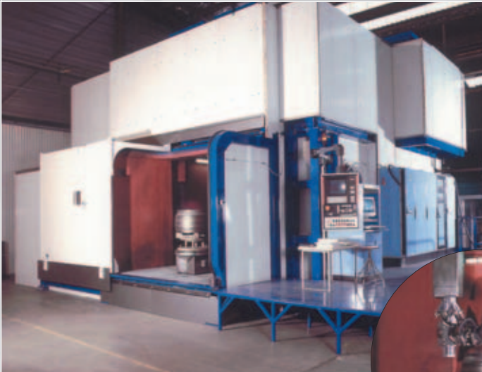
Shot peening machine for engine parts CNC NUM 1060 – 10 axis
