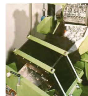
Drum magnet with de-magnetization tunnel
