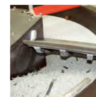
Gentle "cascade" drop behind separation flap: Prevents damage of delicate parts
