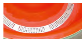
Channel screen – removal of wooden chips
