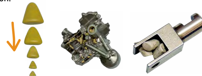
Linear separation unit with vibratory motors
