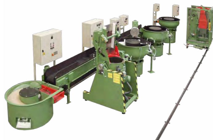
Parts loading: Load system movable on rails with integrated vibratory feed hopper conveyor belt for collecting finished parts and transferring them to a vibratory dryer
