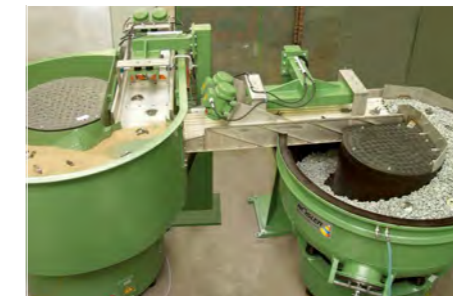
Linear separation unit with vibratory motors
