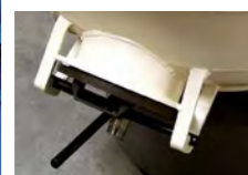
Bottom unload plug with manual locking lever
