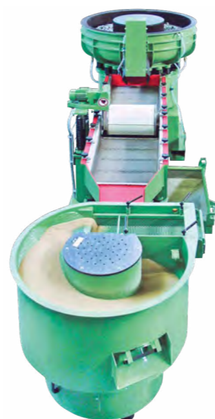
Removal of finished parts and media from work bowl with pneumatic unload gate; external separation with magnetic drum; drying in vibratory dryer
