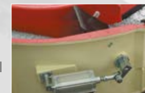
Pneumatically activated separation flap
