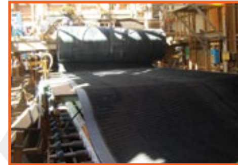
Rubber Drainage Belt for HBF (Horizontal Vacuum Belt Filter)
