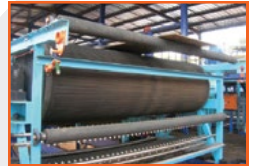
Rubber Drainage Belt for HBF (Horizontal Vacuum Belt Filter)
