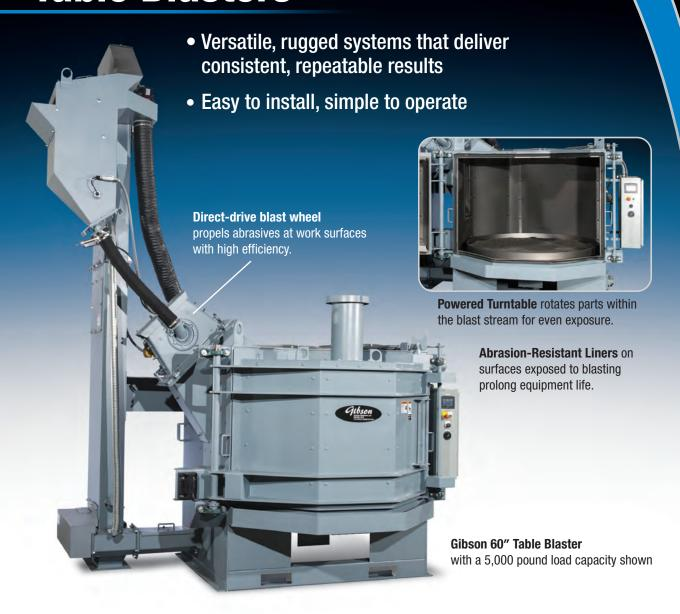
Gibson Table Blasters process parts weighing up to 10,000 pounds with diameters up to eight feet and heights exceeding four. Featuring eleven standard models, Gibson's line of Table Blasters provides the versatility and flexibility to efficiently blast parts ranging from ten-pound gears to heavy fabrications.
