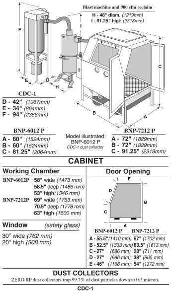
CDC-1 dust collectors come in three sizes; 300 cfm, 600 cfm, and 900 cfm. The cartridges are pulse-cleaned by pressing the manual pulse valve to clear the filter of dust. Dimensions are 34" wide, 42" deep (with motor housing) and 94" high. The MAH is 11 ft for the 300 and 600 cfm units and 12-1/2 ft for the 900 cfm unit.
