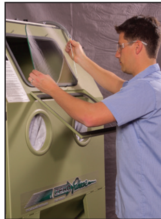
The tilt-out frame makes changing the tempered-glass window a snap.
