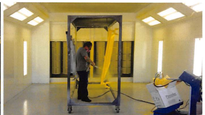
Custom Powder Recovery Booth with hip and sidewall lights
