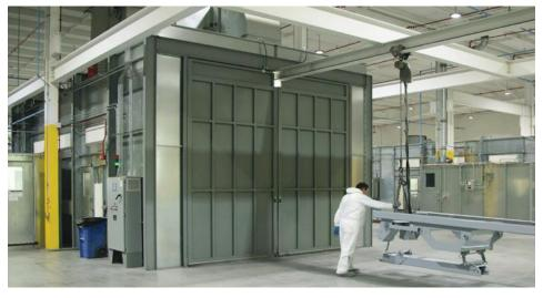
production capacity, manufacturers may also look at isolating priming to a separate booth. Then, the finishing paint booth can be reserved for applying top coat, enabling businesses to move more product through their facility faster. A well-lit, well-ventilated booth allows for a precise application and drying of primers and top coatings.
