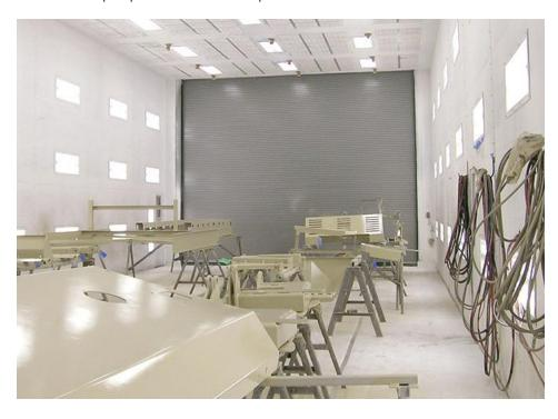
while evenly distributing the air across the booth. High-efficiency filters trap dirt and dust before they enter the booth, allowing for quality paint finishes.
