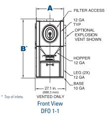
STD DOOR PANEL SHOWN OPTIONAL **EXPLOSION** VENT SHOWN FILTER ACCESS 12 GA  $\mathbf{B}^*$  $\mathbf{B}^*$ DAMPER POWER HOPPER PACK 12 GA 18.9 in. (480.1 mm) ACCESS PΔII PANEL LEG (2X) 12 GA BASE 1.0 in. (25.4 mm) 27.1 in. —— (688.3 mm) VENTED ONLY Front View Left Side View
