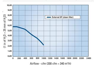
DFO 2-2 2.2kW 50Hz with 8" (203.2 mm) inlet duct (clean filters)
