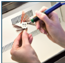
Epoxy removal from probe rings
