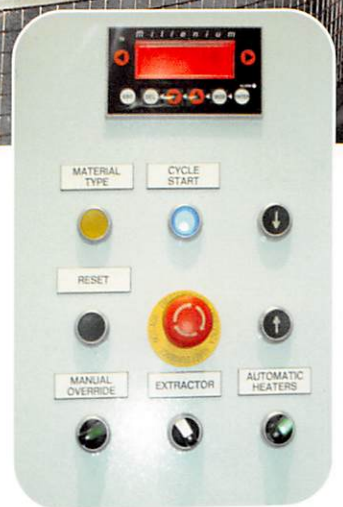
Master Control Panel
