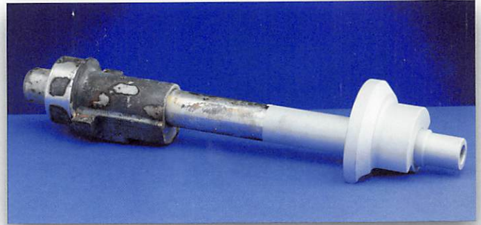
Balance shaft cleaned after braising
