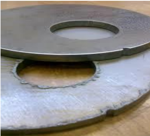
Typical steel plates with Slag and Dross:
