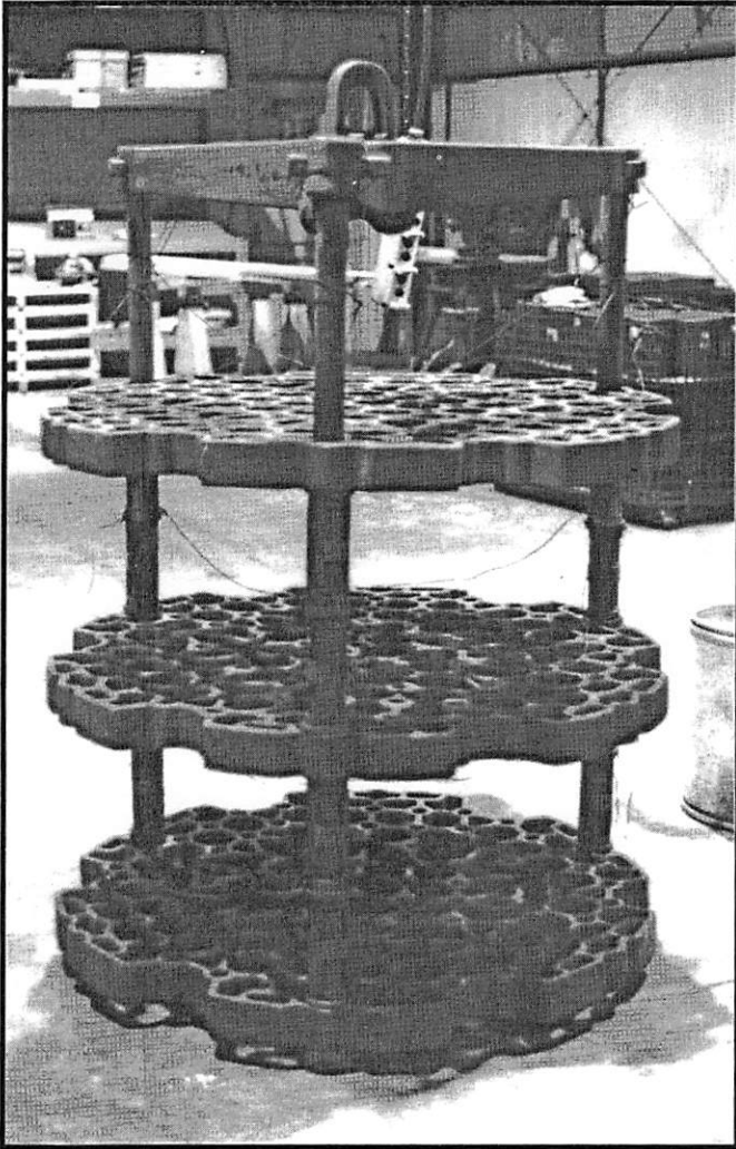
Cast HUCB Alloy 3-Post Lifting Fixture for Pit Carburizing Furnace
