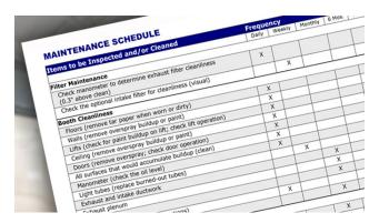
It is best to work with your paint booth manufacturer or filter supplier to design an effective replacement schedule for your filters. This schedule should balance your filtration and paint booth performance needs with the costs — and savings — of more frequent filter replacement. At GFS, we have an expert team of parts and filters sales representatives who can help with all your filter needs.
