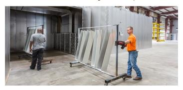
The decision on whether to choose a gas or electric oven typically comes down to whether a manufacturer needs an electric heater for low-temperature applications or only needs a small oven. If not, a gas oven is generally better in the long run.
