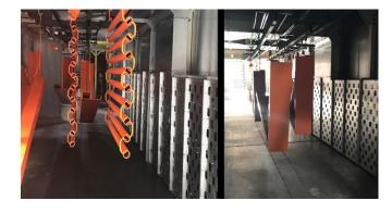
In 2018, JAS Powder Coating of Fort Lauderdale, Florida, replaced their existing gas oven with a 34-footlong, gas-powered Batch Process Oven from Global Finishing Solutions (GFS). Over the past year, they have increased their throughput by 150 percent and decreased their fuel cost by \$7,000. This shows that increased efficiency and cost savings can be realized even when comparing gas ovens.
