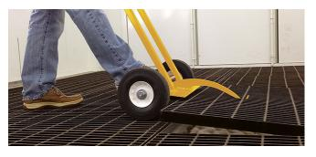
If you have a downdraft booth, lifting heavy floor grates to change exhaust filters can be a time-consuming and exhausting task. To make this process easier, GFS developed the Grate Lifting Tool. This handy tool has a hook on the end for quick, easy lifting and moving of the grate. It not only saves you time but prevents your fingers from getting pinched and your back from being strained.
