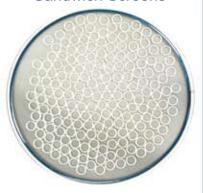
Plastic sliders or rubber balls are sandwiched between a sizing screen and the backup mesh, providing added vibration, dislodging near size particles, and allowing material to flow more efficiently.
