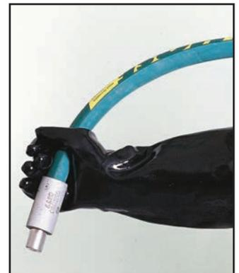
**For tough cleaning jobs, pressure blasting delivers higher abrasive velocity for greater impact intensity, compared to suction blasting, and can increase your production rate by as much as 300 percent.**
