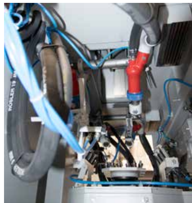
Glimpse into the blast chamber of a Rösler RWS 1200-T1-I4-SAT 1 showing the following details: Blast nozzles, blast turbine, blow-off nozzles and the satellite station with work piece fixture supplied by the customer.
