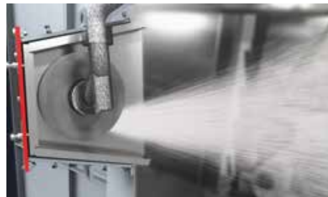
Compared to conventional turbines of the same size, the Gamma 400 G offers a 15 – 20 percent higher shot blast performance.
