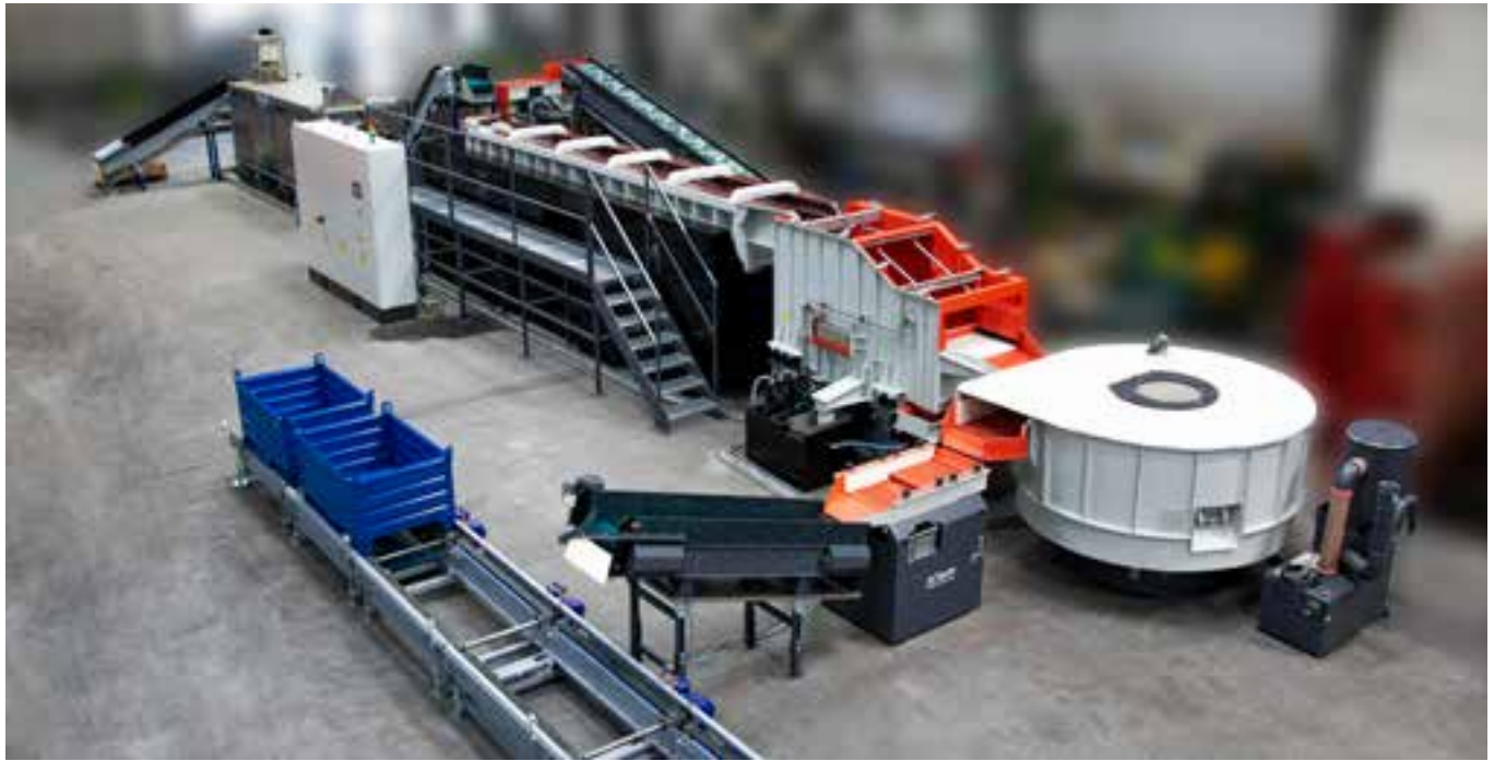
The fully automatic de-oiling/washing and mass finishing system is directly linked to the punch press and allows for continuous feed operation. The only manual operation is the replacement of the full transport bins every few hours.
