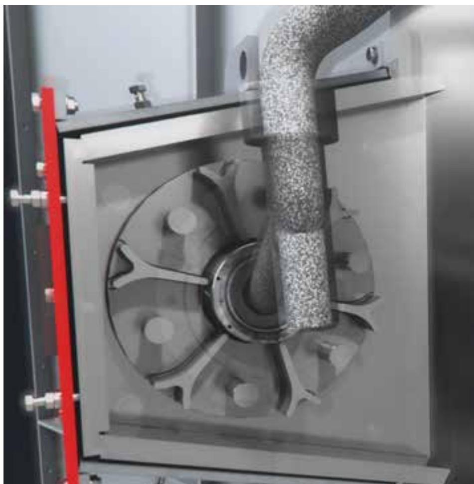
Because of their special "Y" design both sides of the Gamma 400 G throwing blades can be utilized. A special quick change system allows changing the blade set in a turbine in less than 10 minutes.
