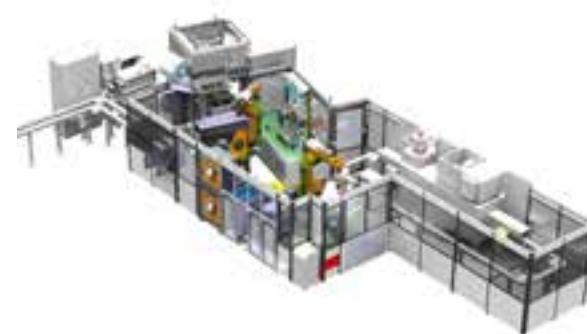
The overall system includes deburring, fine cleaning, quality control, packaging in small load carriers (KLT's) and their transfer to stacking cells.
