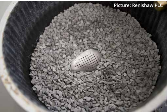
In a 3-stage process the cranial plate implants, mounted to a stationary fixture, receive an extremely smooth surface finish. The cycle time could be reduced from five to less than one hour.
