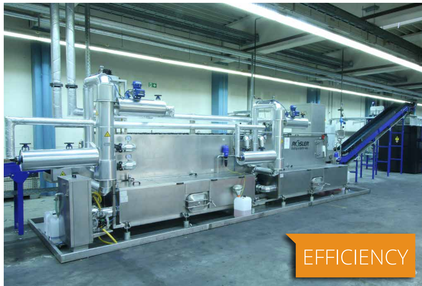
The interlinked solution for de-oiling, mass finishing and deep cleaning of stamped and formed parts for the automotive industry meets not only strict cleanliness requirements but also produces significant time and cost savings.
