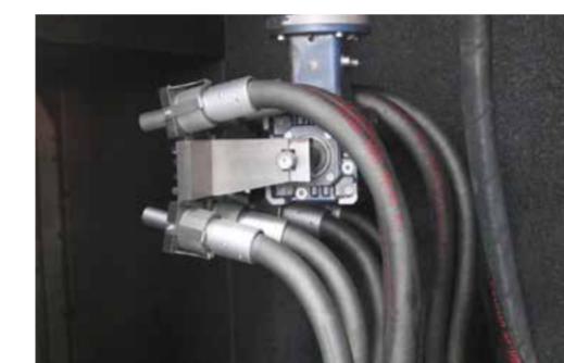
The nozzles can be moved vertically, horizontally and can be pivoted at an angle from 0 to 90°. This guarantees complete coverage of all work piece surface areas. The high efficiency of the pressure blast system results in significant savings in compressed air consumption.
