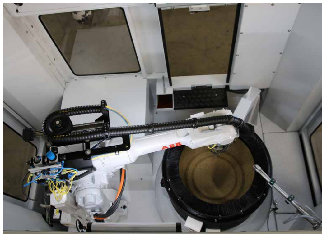
In surf-finishing systems the robot fulfills not only a material handling function but also guides the work pieces through the processing medium during the finishing cycle. This allows treating the complete surface or only specific surface areas of the work pieces.
