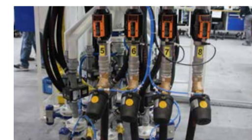
A comprehensive monitoring and control system, which monitors the air volume (orange control unit), ensures the high process safety and consistency required for any shot peening operation.
