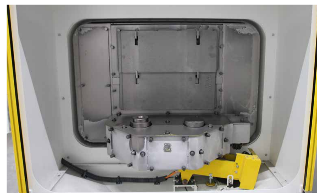
While in one 180° segment, two work pieces can be processed and two work pieces can be loaded/unloaded in the other 180° segment. The RWT design is based on a modular concept that was specifically developed for the peening of transmission components.
