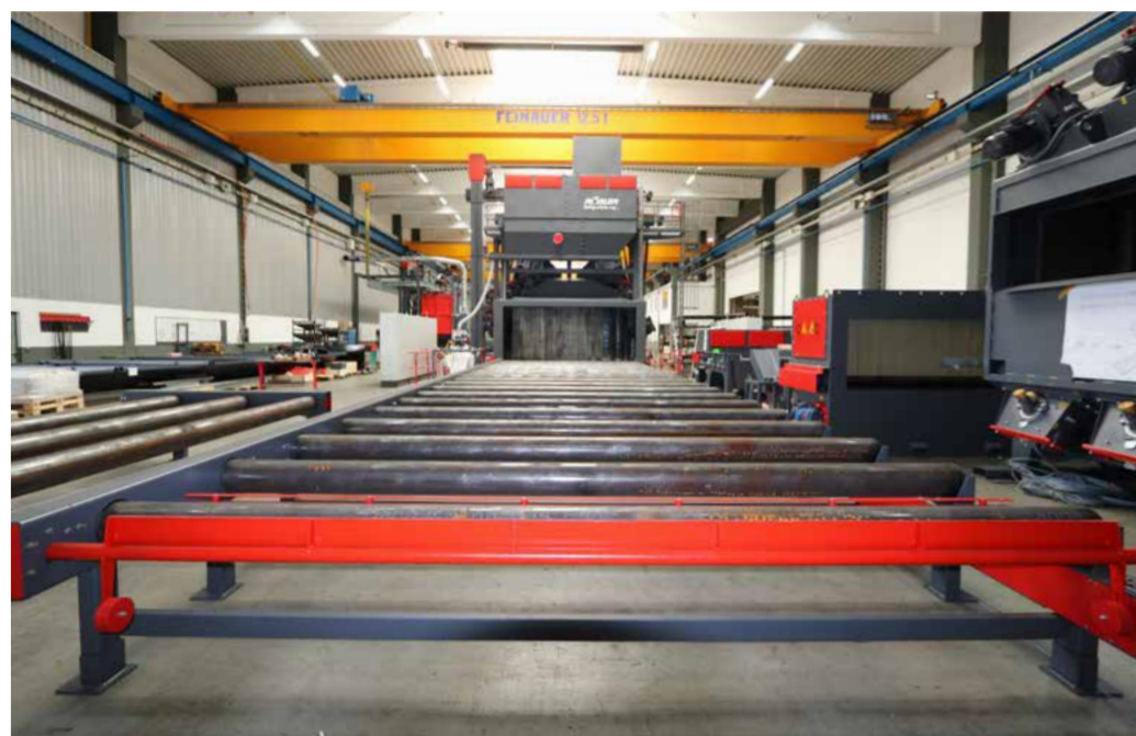
The large RRBK 42/16 L shot blast machine for welding assemblies is equipped with 14 high-performance blast turbines. Their optimum position around the blast chamber ensures perfect blast cleaning results irrespective of the complexity of the shape of the steel weldments.
