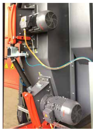
The standard equipment of the RHBE 13/18 includes two energy efficient Gamma 300 G turbines and a blast chamber made from manganese steel. For additional wear protection, in areas directly exposed to the blast stream, the blast chamber is lined with replaceable manganese steel wear plates.
