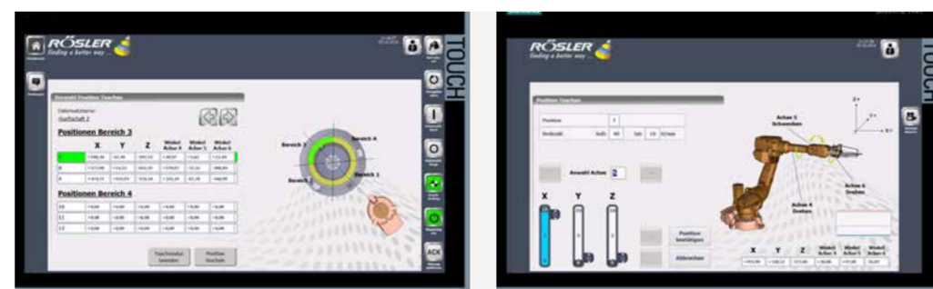
The robot movements can be easily taught with the operating panel without any additional hard- or software. No special robotic experience or knowledge is required.
