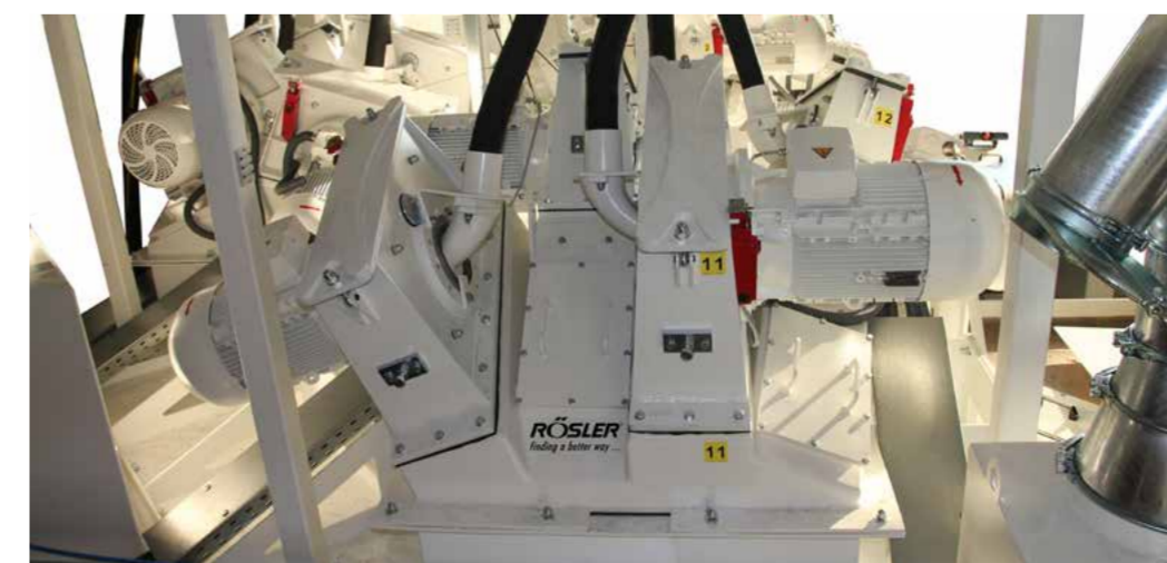
Each of the three blast chambers is equipped with four Gamma G turbines with an installed power of 22 kW each. The turbine location and positioning, which is determined by a computer simulation, guarantees perfect, all-around blast cleaning of the different types of crankshafts.
