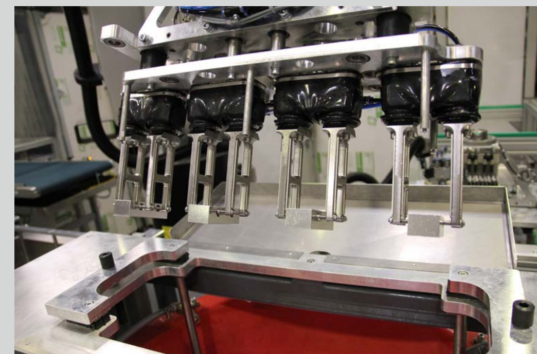
During the HFF process the robot immerses the rotating work pieces mounted to a specially designed gripper into the media agitated by vibration. The finished work pieces undergo a subsequent rinse cleaning process.
