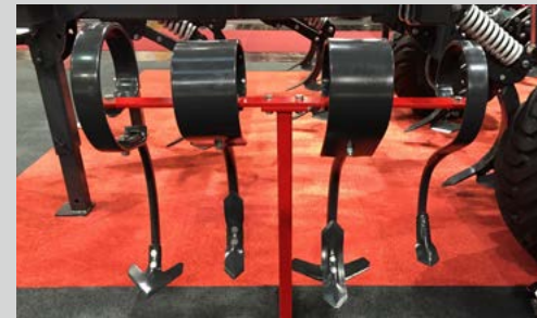
During operation the vibrating tines of the cultivators are exposed to heavy loads. With shot peening their uptime could be significantly increased.
