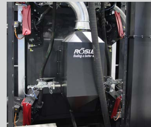
Each blast machine is equipped with eight (8) Gamma® 400 G turbines. Their placement ensures that the individual blast patterns are not overlapping and guarantees perfect blast coverage on the tines.
