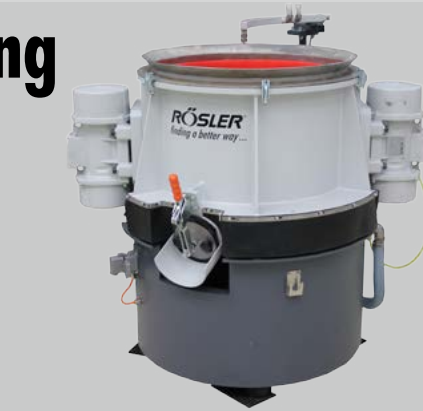
R 150/2 DL vibratory systems allow the effective surface finishing of work pieces with complex geometries in very short cycle times. Bolting the work pieces to the vibrating processing bowl greatly enhances the finishing intensity.
