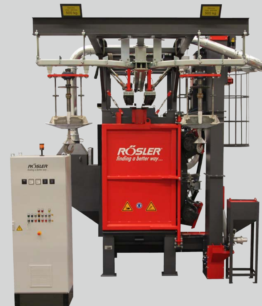
Standard spinner hanger machines, for example, the compact RHBE 11/15 L allow the shot blasting of a wide spectrum of different work pieces. Like with all Rösler turbine blast machines the blast chamber is made from wear resistant manganese steel.
