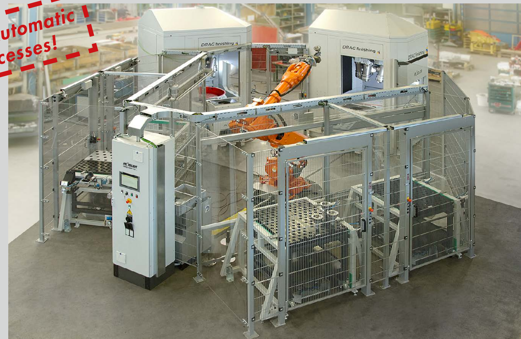
In order to completely automate the deburring of precision components like tool bodies, drag finishers like the model R 6/1000 SF-Auto were completely redesigned to allow robotic loading/unloading of the work pieces.
