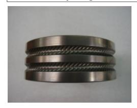
Profiling rollers are utilized to generate a corrugated pattern on the surface of steel products, (i. e. structural steel). Corrugated steel is primarily used in the building industry. Profiling of the sheet metal surface is the final step in the overall manufacturing process.
