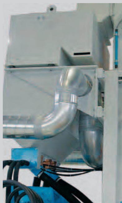
Deflashing medium reconditioning via cascade separator
