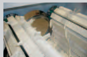
View into the loop belt trough (lamellar-type rubber elements for gentle component transport)
