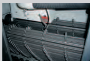
View into the loop belt trough (metal profile) for small parts
