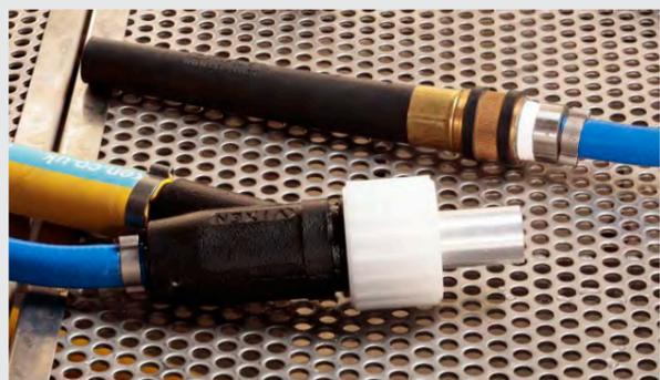
Flexi on/off rinse gun (top) has no external moving parts that could cause obstruction
