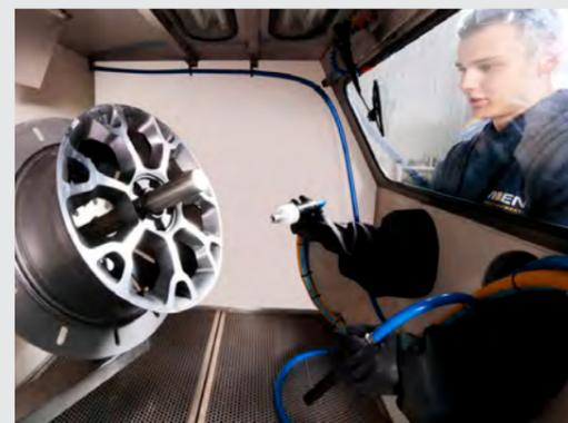
4 After contact with the component, the slurry drains back into the sump and is recirculated.
