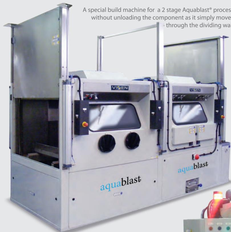
A special build machine for a 2 stage Aquablast® process without unloading the component as it simply moves through the dividing wall
