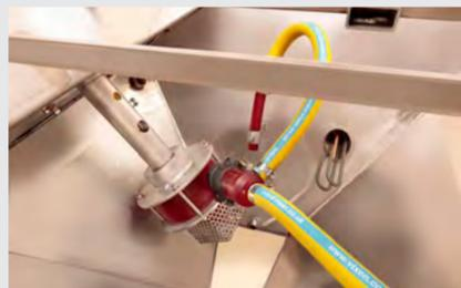
2 Delivery of the slurry to the hand-held nozzle is via a glandless polyurethane pump and hoses within the machine.
