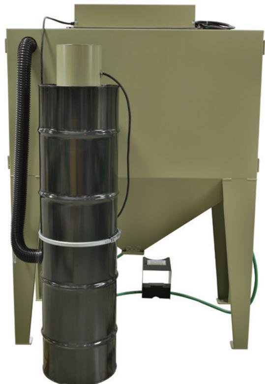
The INEX™ 3048R is a suction-blast-style light-duty intermittent-use cabinet with a 300 cfm reclaimer and reverse-pulse dust collector. The addition of a reclaimer improves blast quality by ensuring only clean, properly-sized blast media is being used. It comes with a No. 5 BNP Gun and a 5/16-orifice ceramic nozzle but can be fitted with longer wearing tungsten or boron-carbide nozzles when aggressive blast media is used.
