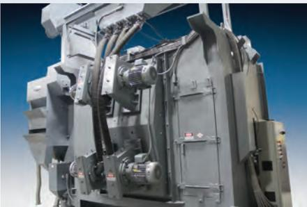
High-capacity blast machine performs both **Table** and **Spinner Hanger** operations, providing the versatility to meet various customer needs.
