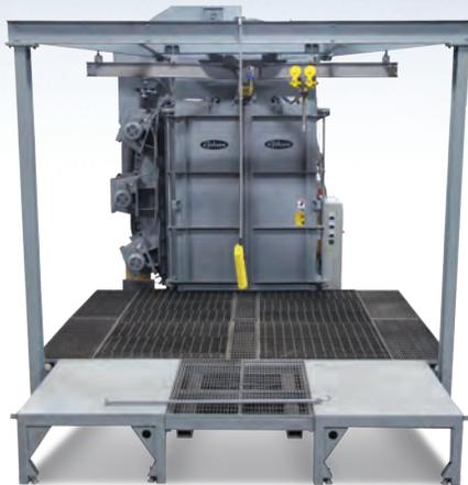
Gibson offers single chamber systems for heavier, harder to load parts. Optional Y-track upgrades branch two rails so one fixture can be loaded and unloaded while parts on the second fixture undergo blasting.
