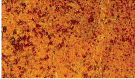
**KEY:** Steel where all mill scale has flaked off and complete rusting has occurred.
