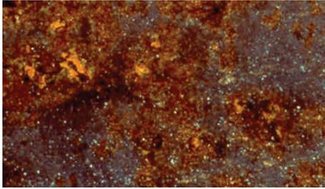
**KEY:** Steel where mill scale has started to flake and light rusting occurs.
