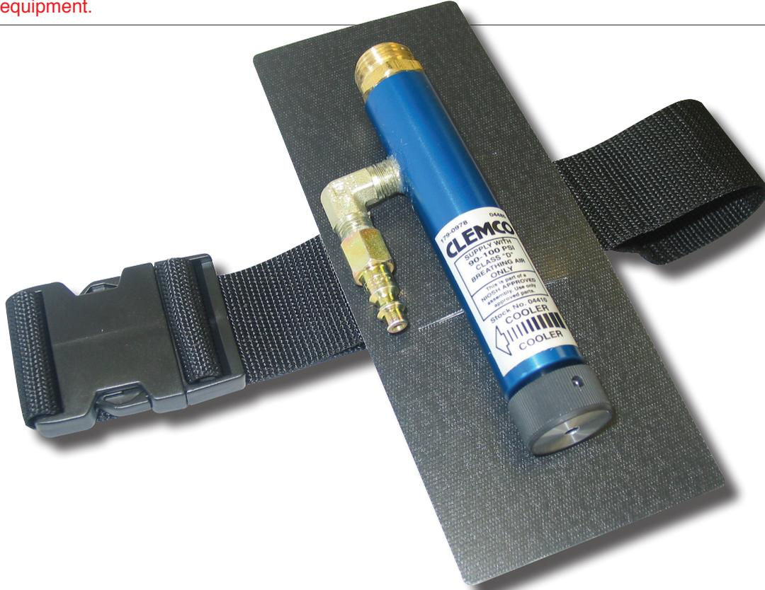
**OVERVIEW**The Clemco Cool Air Tube (CAT) allows the blast operator to control the temperature and volume of air to a Clemco Apollo HP Type CE continuous flow supplied-air respirator within a preset range and to cool incoming compressed air by as much as 50° F
