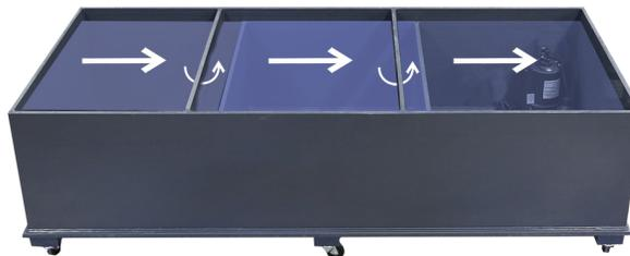
**How It Works-** Water that drains from the table into the sludge tank enters the first compartment. As the compartment fills the water travels through the baffling to the second and third compartment where it is pumped out.
