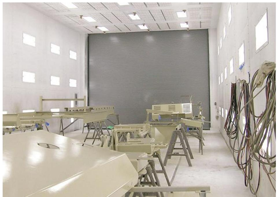
while evenly distributing the air across the booth. High-efficiency filters trap dirt and dust before they enter the booth, allowing for quality paint finishes.
