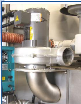
**2) DRYING STAGE** After the wash and rinse stages, the parts dried with a high velocity (15,000ft/min) blast of hot (typically 260 F) air. For drying, the machine is equipped with a regenerative blower (5 HP for CJ-2, 10 HP for CJ-4), a low watt density air heating system (12.8 kW for CJ-2, 21 kW for CJ-4), and a steam exhaust blower.
