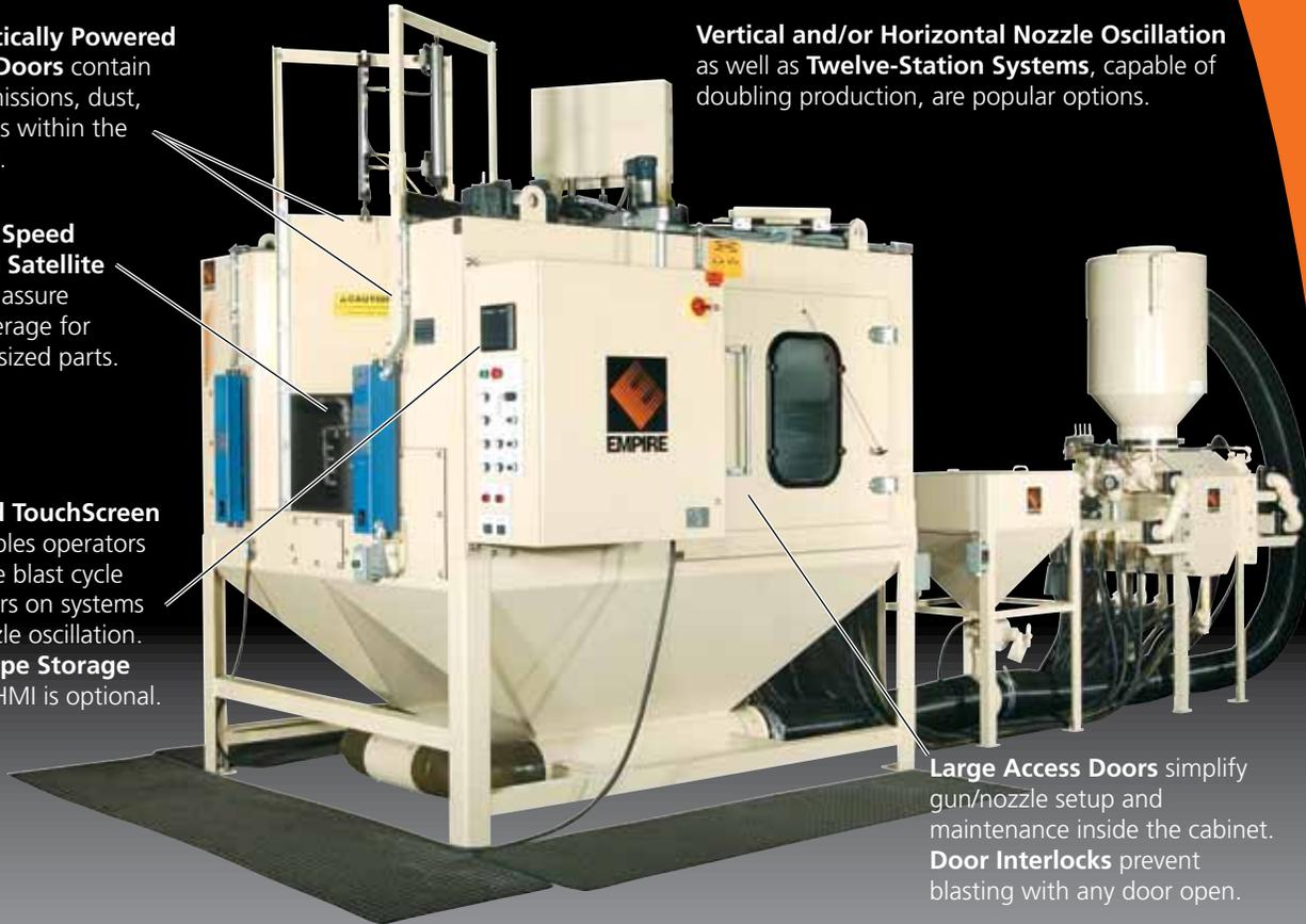
**Large Access Doors** simplify gun/nozzle setup and maintenance inside the cabinet. **Door Interlocks** prevent blasting with any door open.
