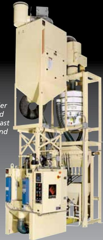
*Shot-Peening Turntable includes a vibratory classifier plus closed-loop control and monitoring of shot flow, blast pressure, rotation speeds and nozzle oscillation rates.*
