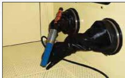
High-intensity lighting, a venturi blast nozzle with lightweight blast hose, and abrasion-resistant operator gloves boost productivity.
