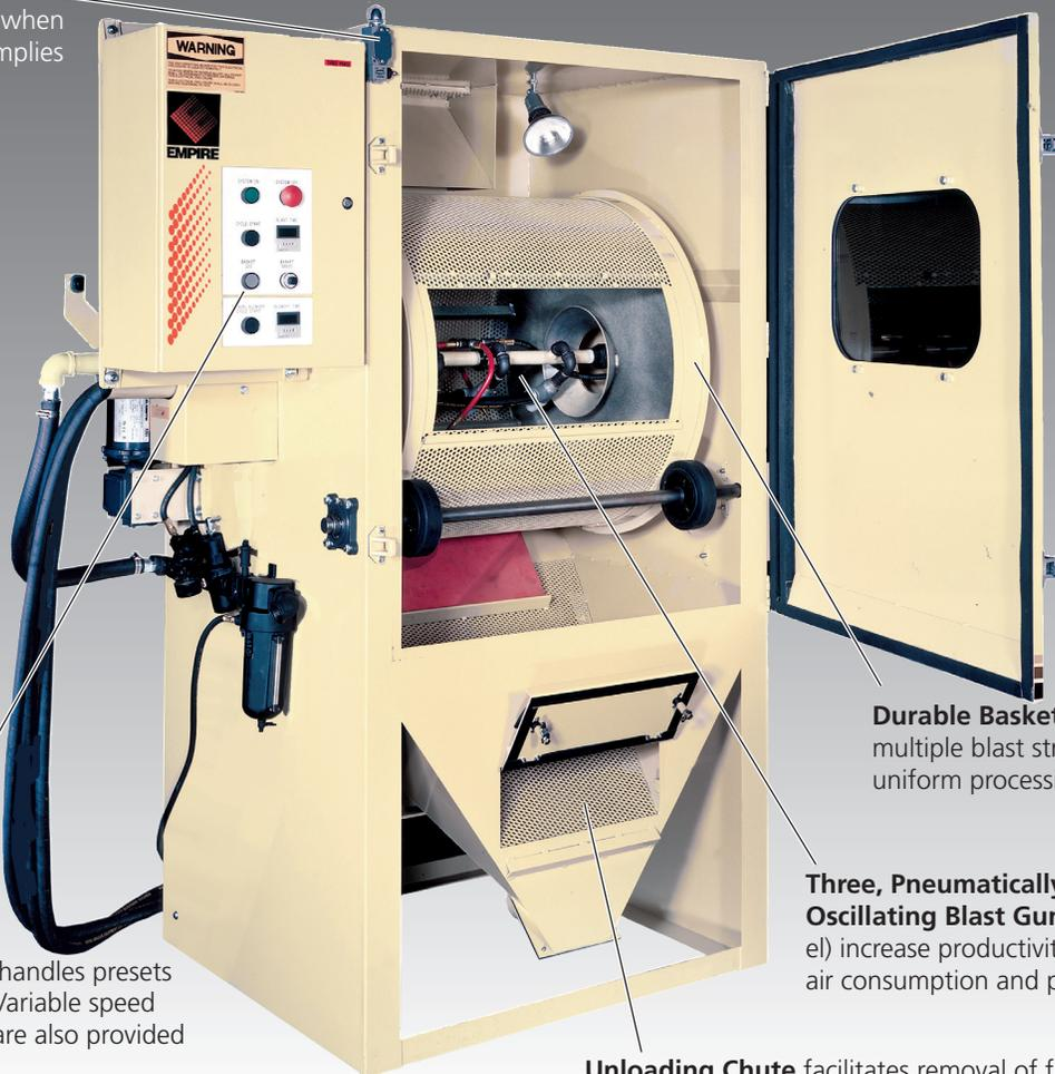
**Precision Timer** handles presets of any duration. Variable speed and jog controls are also provided for the basket.
