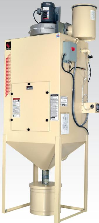
**Standard Features:** • Quick-release basket door • External blow-off gun • Door/blast interlock • Easily unloaded hopper door • Precision timer • 1/3-hp., DC variable drive (1 to 5 RPM) • 3-phase fan motor • Heavy-duty conveying hose • Lined, tunable reclaimer • 1" piping with general purpose filter, gauge and pressure regulator • Electrical control box • Two, 90-watt interior lights • Easily accessed media hopper • Observation window • Cabinet and dust-collector leveling bolts
